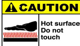
**Caution: Surface May be Hot.** Ensure PTO is off and unit has cooled before servicing.
